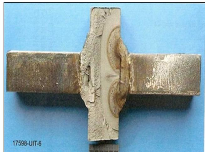
Figure 6. Fatigue crack from root and into main plate of a pre-fatigued and treated test piece.
