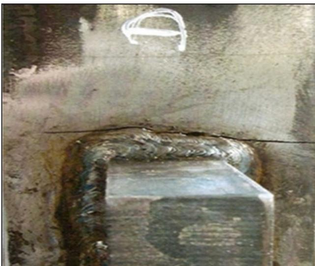
Figure 5. Fatigue crack from weld toe and into main plate of an as-welded test piece
