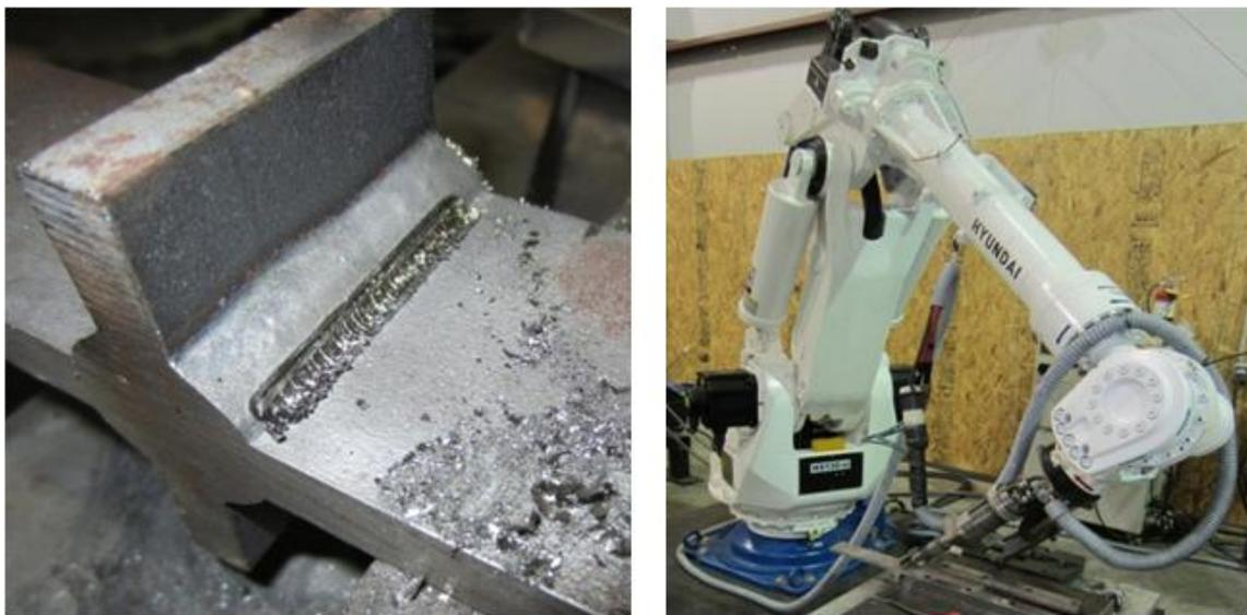
**Figure 4 – Over-Treated Specimen (Left), and Robot (Right)**
