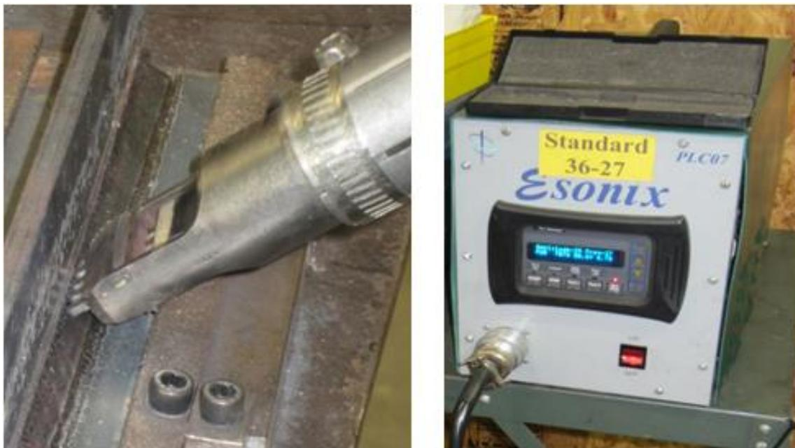
**Figure 1 – Ultrasonic Impact Treatment Equipment**
